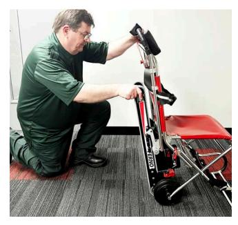
Push track towards chair to close the push-to-close latches and attach the track to the frame
