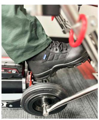
3. With the Track module laid on the ground still attached to the chair axle, straddle the track behind the chair bring your foot in under the chair and using your heel of your foot, pull back on the RED release handle on the Track module to disengage the axle locking mechanism and then lift the Chair out of the axle locking mechanism.
