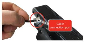
Connecting the cable to the connector port
