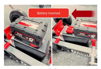
Battery attached to motor
