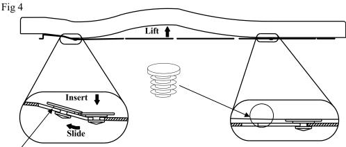
**Note:** The pegs in the Head Rest Panel should not reach the end of the slot when the Head Rest is down. The gap left allows movement when the Head Rest is raised.
