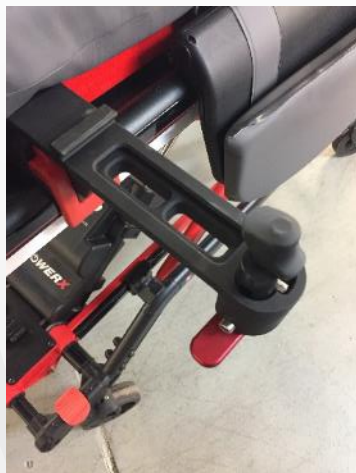
Attach brackets to sides of PowerX on interface rail
