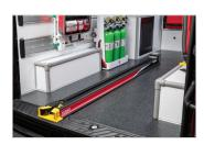
**Straight in-track design** eliminates the need to steer the cot when loading and unloading
